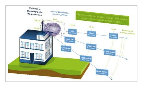
The calculation of the safety volume is defined by a parallelepiped as shown in the figure, the lengths of which are defined from the data for this antenna.
