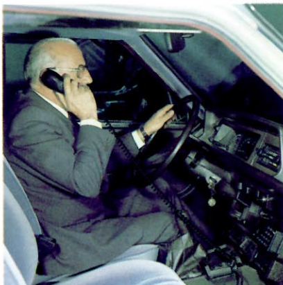
Automatic mobile telephone (T.M.A.).
