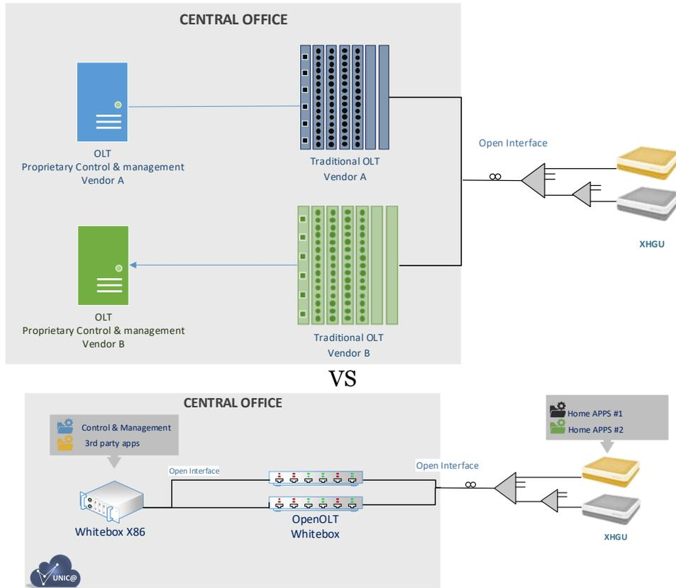
**FIGURE 6:** Distributed Fixed Traditional VS Open Access architecture
