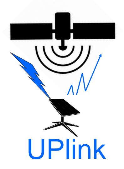
Uplink: It is difficult for satellite networks to get a good signal from small devices. WE are testing bonding of different devices/links/networks to get more uplink. WE have as well plans for local breakout, so that local traffic stays local.
