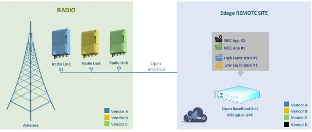
FIGURE 4: Distributed mobile Traditional vs. Open Access architecture
